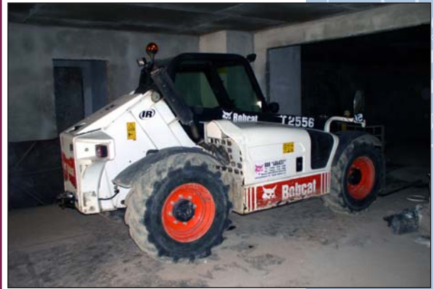
Fig. 16. «The Alfa-Arbat-Center» multifunctional complex in Moscow. Facing materials transported over the ramp to the -3 rd storey with small-size loaders while excavating the 5 th tier of the pit.
